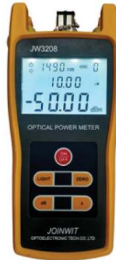
Gambar 5.6 Optical Power Meter Sumber: Arif Muttakin (2022)
