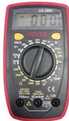
Gambar 5.4 Multimeter Digital Sumber: Arif Muttakin (2022)
